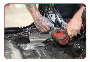
Mark the three holes that need to be drilled. Drill the three holes that bolt MB3032-06 to the tub floor to allow a 3/8" bolt to pass through.
