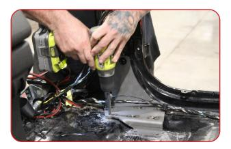
After drilling bolt MB3032-06 back to the place and fasten using the two factory bolts that attach to the B-pillar and the three 3/8" bolts that bolt through the tub. The factory wiring harness should be above the plate and not pinched between the B-pillar mount and the body.
