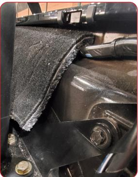
Fasten the assembly MB3032-09 and MB3032-10 to the Jeep tub using the provided 3/8" hardware for the holes that were drilled and the factory hardware.
