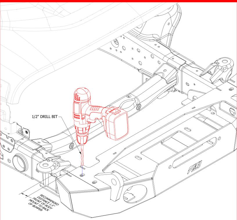
USE BUMPER TO MARK HOLES TOP AND BOTTOM REMOVE BUMPER AND DRILL HOLES DO NOT DRILL THROUGH TOP AND BOTTOM AT THE SAME TIME REV
