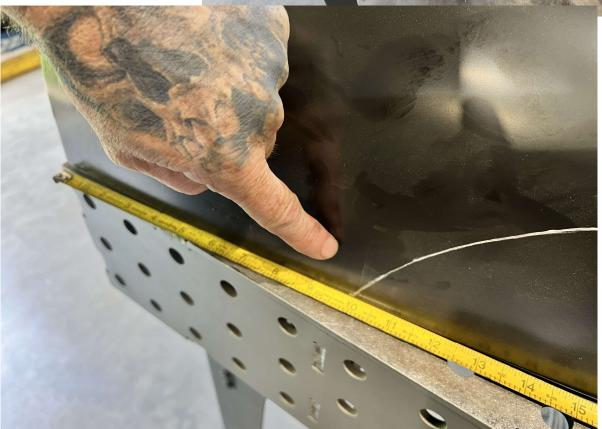
The point where the cut line meets the bottom of the hood should measure 10 inches. Adjust your cut lines (if neccessary) to meet this 10" measurement.
