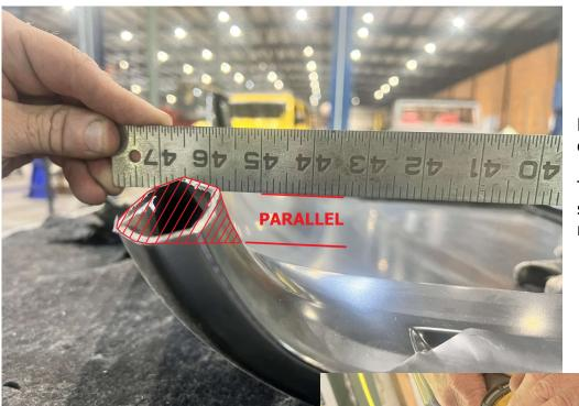
Flip the hood over. Use a straight edge & mark material to be removed.
