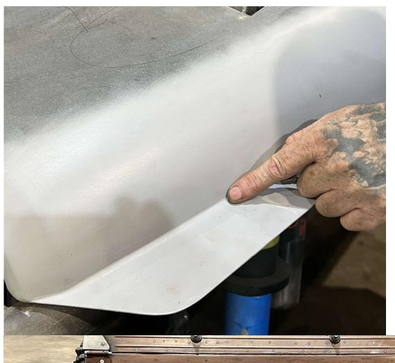
Add seam sealer & bondo to surfaces. Sand & blend. Prime & paint surfaces.
