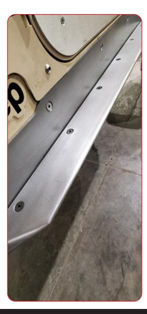
Loosely fasten MB1136-A to MB1136-08 with six (6) 3/8"-18 x 1" flathead socket cap screws into the barrel screws installed earlier on MB1136-08.
