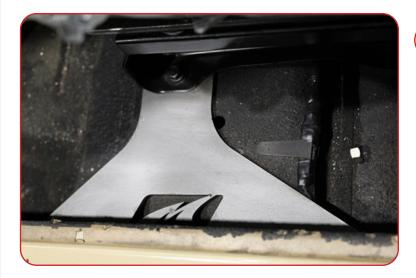
Install MB1136-09 by first removing the front two seat bracket bolts. Slide MB1136-09 between the seat bracket and jeep floor. Re-install the two bolts into the seat bracket.
