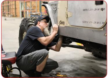
8 Attach the remaining top row hardware on MB1136-07 using 3/8"-16 x 1" flathead socket cap screws and 3/8"-16 Nylock nut and 3/8" flat washer.
