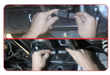
Disconnect rear bumper wiring harness at two (2) locations. Move the red tab outwards then press on the connector to disconnect.
