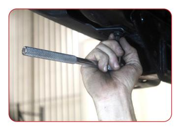
Using a T-50 Torx socket, remove two (2) M10 bolts located on the underside of the hitch cross frame member.
