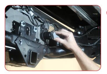
**36** Connect the trailer 7 pin wiring connector.
