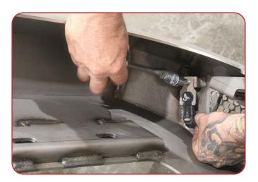
If equipped, install park sensors by placing the sensor in the hole then position MB2117-01 Sensor Retainer plate over the back side of the park sensor. Fasten using #10-24 x ½" long Hex Button Screw (4 places total)
