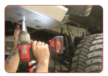
With all fasteners loosely installed, measure the gaps on each side between the body & the bumper. Adjust left or right as needed. Tighten all fasteners including the Frame Rail Brackets.
