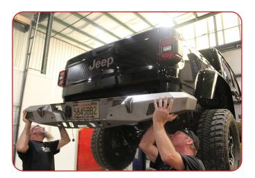
With the bumper assembled & wiring in place, grab an assistant to help you lift the bumper by supporting each end & align the four (4) threaded studs with the mating plates in the rear frame. Loosely fasten using four (4) 7/16" Flat Washers & four (4) 7/16" Hex Flange Nuts. Do NOT tighten nuts yet.
