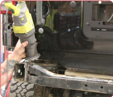
Mark, cut and remove factory rear crossmember and body mounts Remove rear body bolts & nuts
