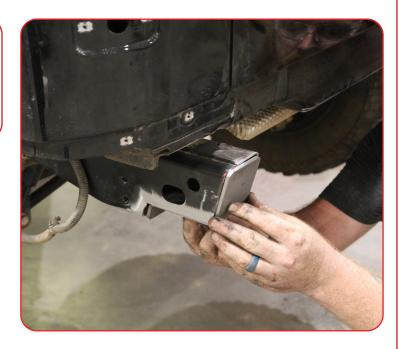
Tack end cap into place and check fitment, then fully weld on end cap
