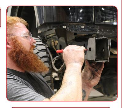
**9** Cut the frame on the marked lines
