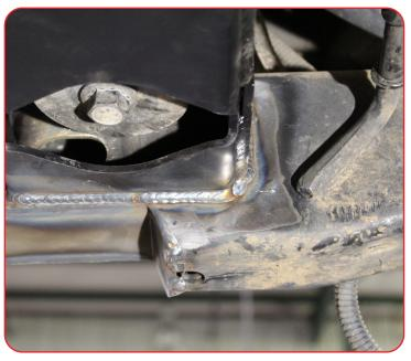
Install bumper using 2 factory bolts on each side of the frame plus three supplied bolts into the crossmember
