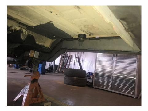
This TJ has a 1.5" body lift so we only had to cut the tub a small amount. You can see where we notched the body just below the tail gate. This kit will work without a body lift but you will need to cut more in this area.
