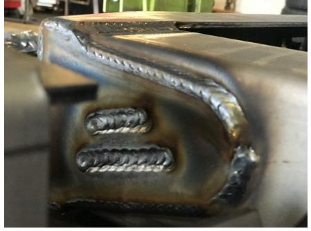
Next reinstall the back half onto the Jeep and weld the new frame rails to the factory rails.
