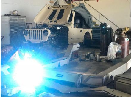
Be sure to test fit the frame rails during the process to ensure nothing moves. Remember it's better to check and be sure then to rush things. You will need to weld the reinforcement end caps that connect the frame rails to the bumper.
