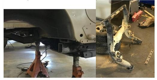
This will allow us to slide on the first part of the Motobilt Jeep TJ back half kit. The new frame rail sections come welded and ready to slide over the frame rails.
