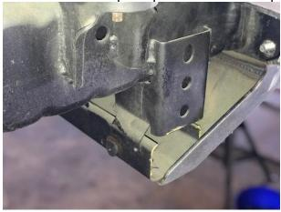
You can see how the crash bar needed to be trimmed on the ends so that the skid plate would clear. 2012 + JK's will need to remove the factory vacuum pump bracket from the frame rails and install a vacuum pump relocation bracket. PN (MB2060)
