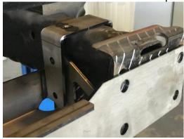
A 7/16" x 1" bolt is used on all of these holes. The hole on the top portion of the bumper will line up with the top hole on this bracket that already has a threaded bung welded into it.
