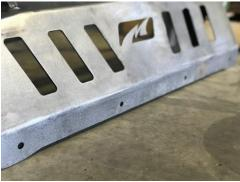
There are 4 bolts 3/8" x 1" that attach the bottom portion of the skid plate to the crash bar.
