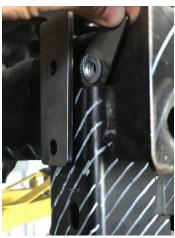
A set of pliers can be useful to hold the end of the flag nut when installing the 7/16" x 1" bolt.
