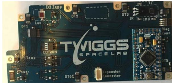
**Figure 2: TSL Primary Payload Board**
