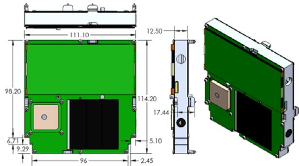
Figure 6: ThinSat Dimensions in Millimeters
