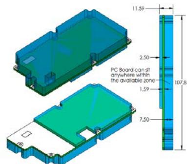
Figure 5: mechanical drawing of the student payload
