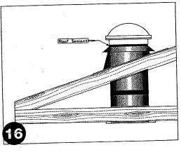
[14] Fasten flashing to the tube assembly with 4 #8 x 3/4" sheet metal screws provided in kit. [15] Caulk around the tube, at the roof jack and the vertical seam of the tube. [16] Apply the storm collar to the tube, just above the roof jack flashing. Caulk around the top of the storm collar.
