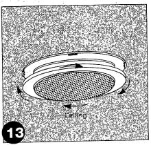
[12] Caulk the tube to the ceiling-mounting ring with white latex caulk provided in kit. [13] Insert the diffuser lens into the trim ring. Center trim ring over trim ring backing plate mounted to the ceiling; rotate clockwise until the trim ring assembly pulls tight to the ceiling.
