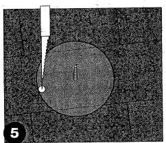
Drill pilot hole inside traced diameter to insert saw blade
