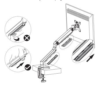
Insert the cable and slide the cable cover down to reattach the cable cover.
