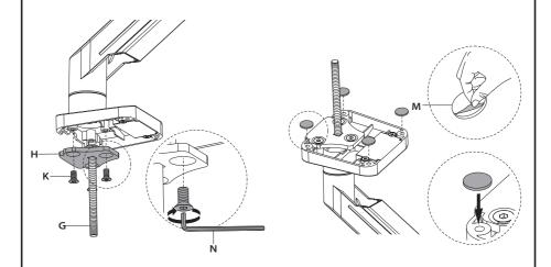
Position stand on desk with long screw through hole, and secure by using the support plate (I) and clamp knob (J) on under side of the mounting surface.
