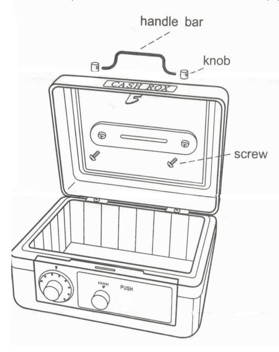
Install Handle using a Screwdriver
