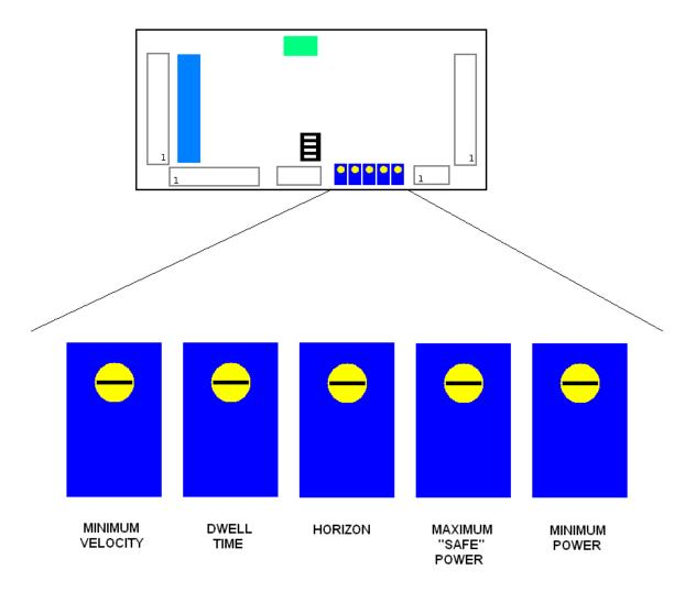
■ The **Minimum Velocity** controls the minimum speed that the beam is required to sweep, in X and/or Y, in order to be considered to be safe. At the factory, Pangolin sets this to around 5 radians per second. Note that the scale of this control (in radians per second) depends on the actual position scale factor of the scanner amplifier being used. Turning this control clockwise increases the minimum velocity (requiring faster scanning in order to be considered safe).
