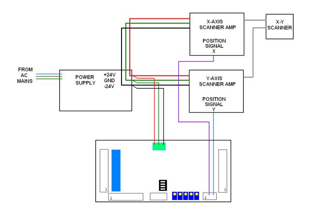
PASS monitors the power supplies that feed the scanner amplifiers. This voltage can be between +/-20 volts and +/- 30 volts. The manor in which you connect PASS to the power supply and to the scanner amplifiers depends heavily upon whether you are using two separate single-axis scanner amplifiers, or one dual-axis scanner amplifier.
