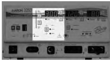
Figure 2 – 3 Controls for the Cut and Blend modes
