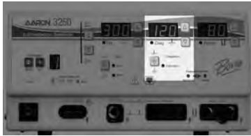
Figure 2 – 4 Controls for the Coag mode
