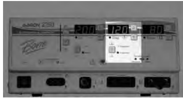
Figure 2 – 3 Controls for the Coag mode
