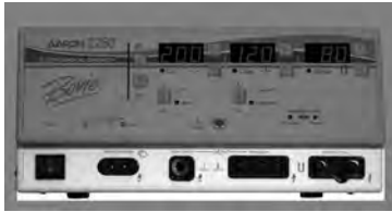
Figure 2 – 6 Location of the unit power switch and front panel receptacles
