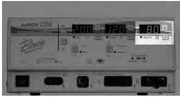
Figure 2 – 4 Controls for the Bipolar mode
