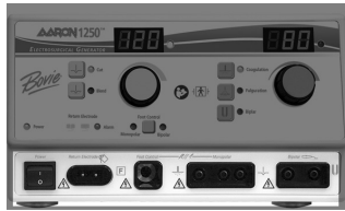
Figure 2 – 5 Location of the unit power switch and front panel receptacles
