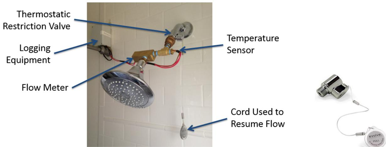
**Figure 1.** ShowerStart Pilot Study Metering Assembly (left) and the ShowerStart Device (right)
