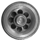
clear valve no blockage
