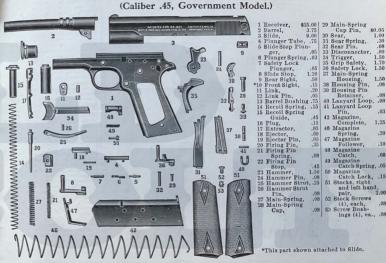
NOTE: When ordering parts, please be sure to give number of pistol and state "Government Model," as parts are different from the previous caliber .45 Colt Automatic Pistol.
