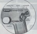
COLT AUTOMATIC GRIP SAFETY, as incorporated in Calibers .22 and .850 Colt Automatic Pistols. (A similar device is also applied to the Calibers .25 and .45.)
