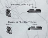
Proper method of sighting, showing "square" formed by Patridge Front Sight in square cut rear: (note strip of light each side of front sight, and position of top in relation to top of rear sight and under bullseye.
