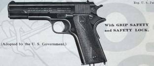
In this model the slide remains open after firing the last cartridge. When reloading the arm in this position, insert the magazine, then press downward the slide stop (to the rear of the trigger as illustrated). The slide goes forward, inserting a cartridge without any movement of the slide by hand. The slide stop is operated by the thumb of the hand holding the pistol.
