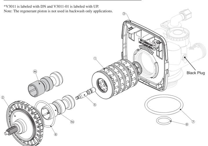
WS1.25CS Drive Cap Assembly, Downflow Piston, Regenerant Piston and Spacer Stack Assembly
