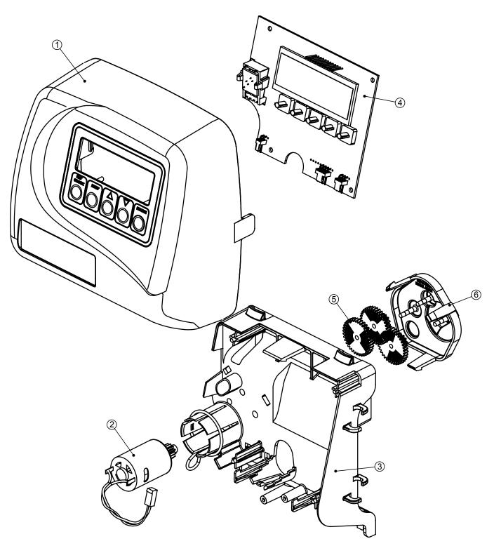
WS1CS Drive Cap Assembly, Downflow Piston, Upflow Piston, Regenerant Piston and Spacer Stack Assembly
