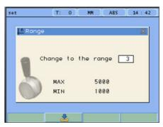
The DRO generates digital outputs in order to be able use an automatic gear change.
