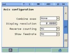
**4- Display feedrate:** Axis feed rate, both in mill and lathe modes. When activating this option ("YES"), the screens shows a window indicating the feed rate of each axis.
