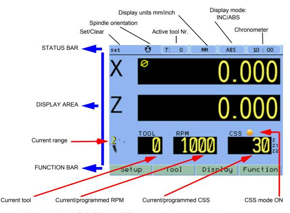
When the spindle is off, the RPM and CSS displays show the programmed values. When the spindle is ON and there is an encoder on the spindle, the RPM and CSS displays will show the current value; but if there is no encoder, they will show their theoretical values.
