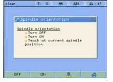
It takes the value of the current spindle position as the preset position to stop
