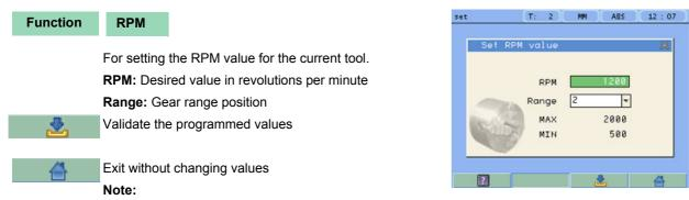
The preset value must be between the minimum and the maximum rpm for the selected range (gear). Setting the RPM value turns the CSS mode OFF.
