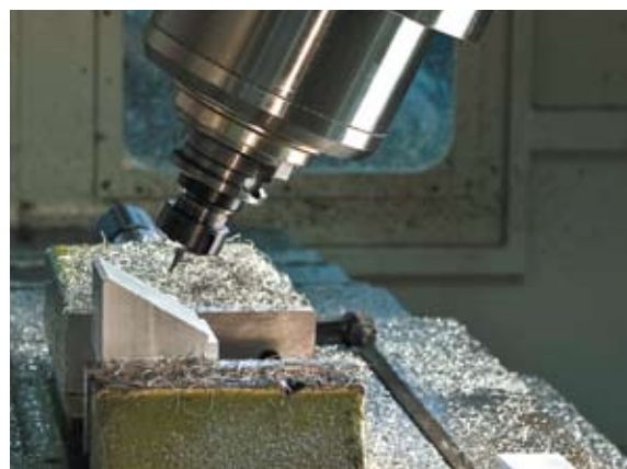
Work in inclined planes
