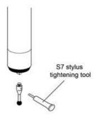
To fit a stylus to a Renishaw touch-trigger probe, insert the correct threaded stylus or stylus adaptor into the stylus mount and tighten the stylus securely using the S7 stylus tool provided. Tightening the stylus by any means other than the stylus tool provided (e.g. spanners, drill bits, etc.) may cause internal damage to the probe mechanism.
