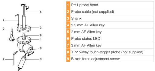
The A-axis may be swivelled through ±115° and locked in position using the 3 mm AF Allen key [7] supplied. For instructions on how to move and lock the A-axis, see 'Moving and locking the A-axis'.
