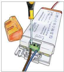
**6** Wiring the power supply to the mains power lead
