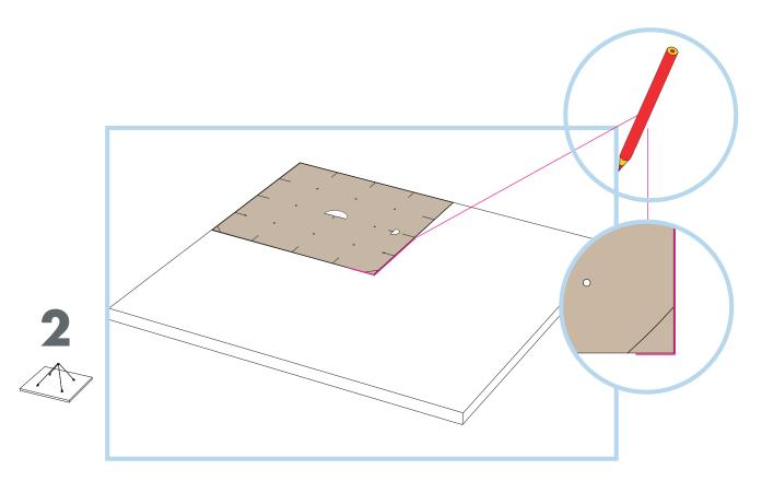
Place the template into the corner shown, mark a line from the outer edge up to signify the middle of the panel.
