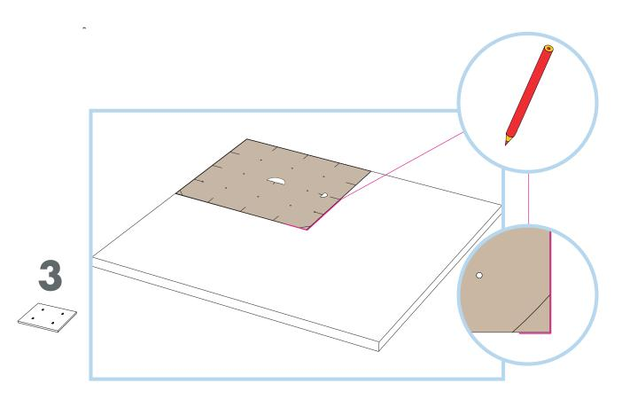
On the rear of the Solo, mark the centre point by aligning the corners of the template with the edge of the Solo as shown.
