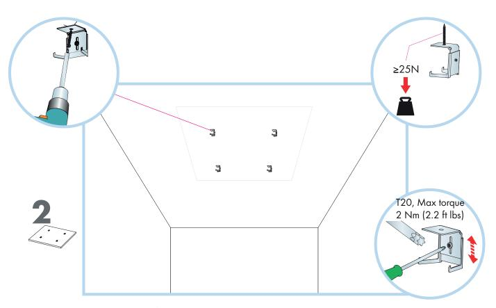
Screw the top of the bracket into the ceiling at the points already marked
