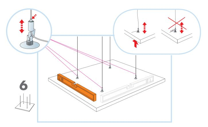
Attach the Adjustable Wire Hanger hooks to the Absorber Anchors and adjust by depressing the button on top of the hook, which enables the hook to travel up and down the wire. All wires should be under tension.
