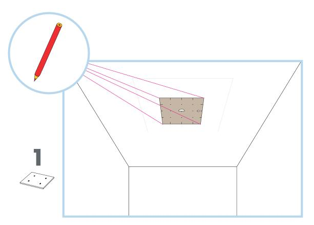
Use template to mark out the 4 fixing positions on ceiling using the points shown above.
