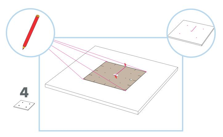
Using the line made in the middle of the panel, line up the template and then mark each corner.
