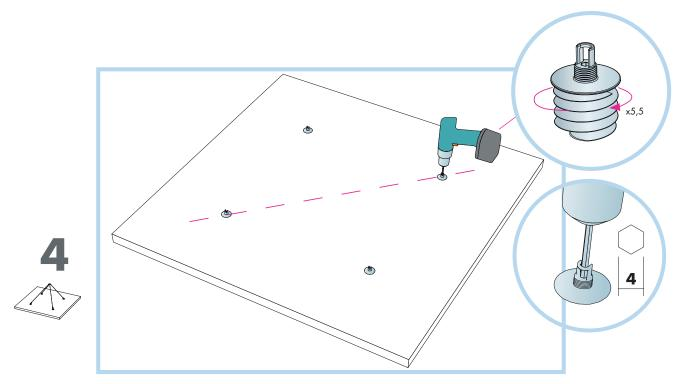
Position the Anchors into the panel on the four points marked, do 5.5 rotations of ensuring the opening of the eye is facing inwards. Shown in the above picture.
