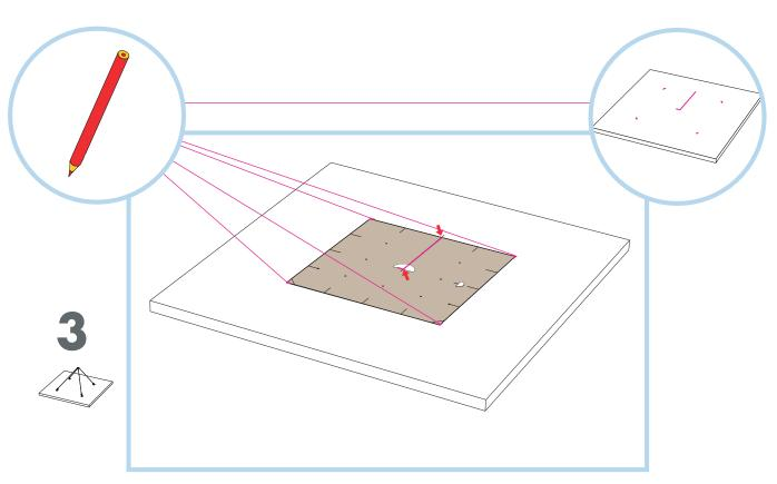
Using the line made in the middle of the panel, line up the template and then mark each corner.
