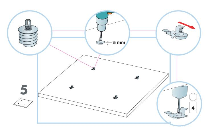
Using a 4mm hexagon tool, fix the 4 Absorber Anchors into points made, leaving 5mm distance between the panel and the head of the anchor. Slide the arms of the bracket under the head of the anchor and fasten with a screw driver.
