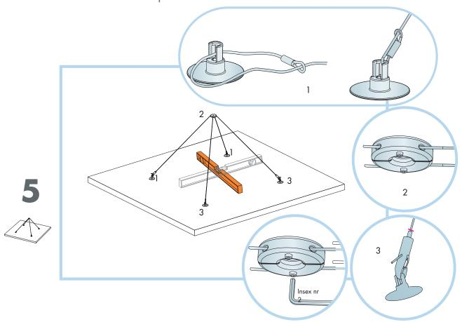
Feed the end of wire through the eye of the anchor shown in diagram 1. Then feed the wire through the One-Point fixing shown in diagram 2. Slide the hook onto the wire Absorber Anchors and adjust by depressing the button on top of the hook, which enables the hook to travel up and down the wire and secure to anchor.
