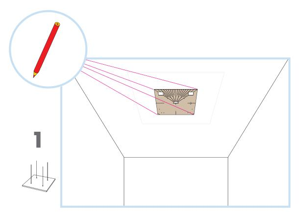
Use template to mark out the 4 fixing positions on ceiling using the diagram above.
