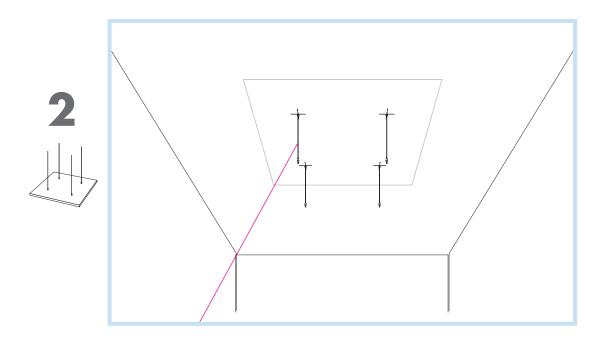
Screw ceiling part of Wire Hanger Kit into ceiling positions marked. Attach wire and hook.
