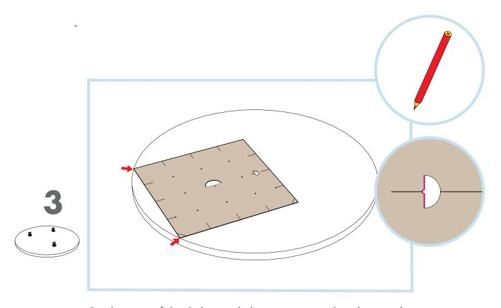
On the rear of the Solo, mark the centre point by aligning the corners of the template with the edge of the Solo as shown. For 1200 circle, align to corners of template, for 800 circle, align to curved line.
