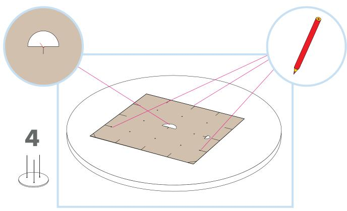
Using the line made in the middle of the panel, line up the template, then mark out the 3 fixing points as shown above.
