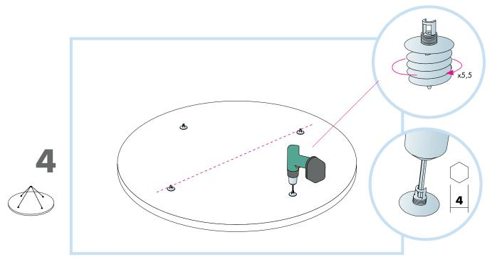
Position the Anchors into the panel on the four points marked, do 5.5 rotations of ensuring the opening of the eye is facing inwards. Shown in the above picture.
