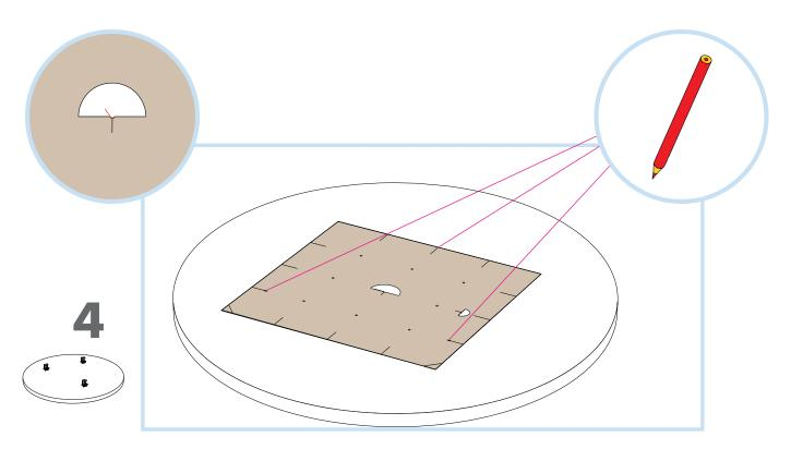
Using the line made in the middle of the panel, line up the template, then mark out the 3 fixing points as shown above.
