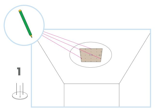
Use template to mark out the 3 fixing positions on ceiling using the points shown above. It should be an equilateral triangle with the points 520mm apart.
