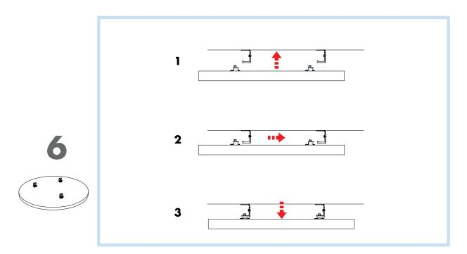
Lift the panel up onto the bracket and slide in place.
