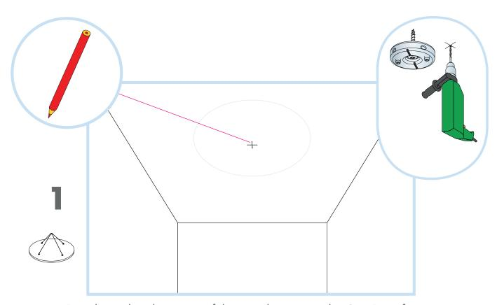
Decide on the placement of the panel, ensuring the One-Point fixing is screwed into the central point on the ceiling.
