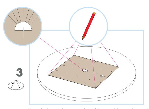
Using the line made in the middle of the panel, line up the template and then mark each corner.
