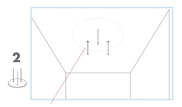
Screw the cup part part of Wire Hanger Kit into ceiling positions marked. Attach wire and hook.
