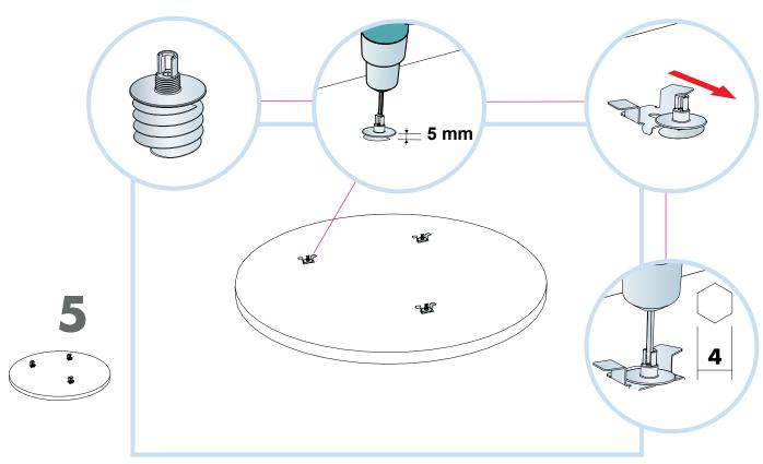
Using a 4mm hexagon tool, fix the 3 Absorber Anchors into points made, leaving 5mm distance between the panel and the head of the anchor. Slide the arms of the bracket under the head of the anchor and fasten with a screw driver.
