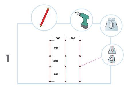
Mark on the wall where you want your baffles to sit, please note the anchor is 100mm below the top of baffle.
