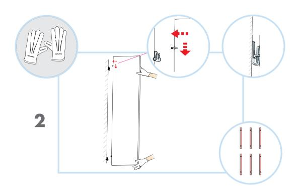
Wearing gloves, slide the baffle hook over the anchor and release down to engage, ensure you are engaging the top and bottom hook in one movement.
