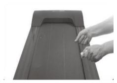
Pull up tightly of the running belt. Then apply the silicone oil to the running board. Start the machine and let it run for 3 minutes without using. It is recommended to do this after every 30 hours of use. This can extend the lifetime of parts.
