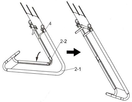
NOTICE THIS SLIDE CAN BE FOLDED UP AND SECURED LOOSELY UNDER THE FRAME TO PREVENT UNAUTHORIZED USE BY YOUNGER CHILDREN. WHEN NOT IN USE PLEASE LEAVE THE RAMP SLIDE FOLDED IN THE STORAGE POSITION AS SHOWN NEXT IN STEP 4.
