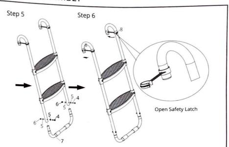
Setp 5. Now that the steps of the ladder are assembled, the final step is to insert the lower frame base onto the ladder rails. Match up the bolt holes and insert the M6x33 bolt with a washer on the backside of rails. Secure with a M6 nut.
