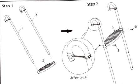
Setp 1. Lay the two curved ladder rails on a clear area. Step should be angled toward front of ladder as shown. Insert one ladder step through the bottom leg of each ladder rail. Slide the step up until it matches the top set of holes.
