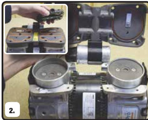
2. Mark the orientation of head plate(s) and remove. Mark the orientation of valve plate(s), remove valve plate(s). Clean valve plates with water based solvent, take care not to scratch valve seats.
