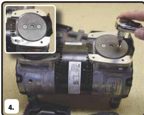
4. Remove screws from cup retainer plate with T15 Torx driver. Discard old cups and retainer screws.
