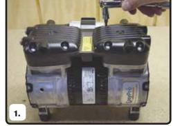
Remove screws from the head of compressor using T25 Torx driver, remove the head
