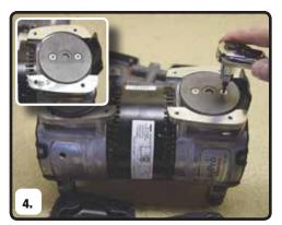
Remove screws from cup retainer plate with T15 Torx driver. Discard old cups and retainer screws.
