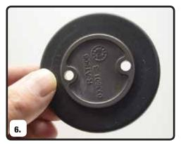
Remove new piston cup(s) from protective cardboard packaging. Set new piston cups onto retainer plate, these parts will sit flat against each other.
