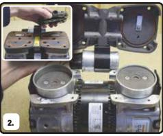
Mark the orientation of head plate(s) and remove. Mark the orientation of valve plate(s), remove valve plate(s). Clean valve plates with water based solvent, take care not to scratch valve seats.
