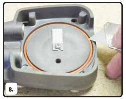
Remove the cylinder o-ring(s) from the bottom of valve plate(s) and install new o-rings.
