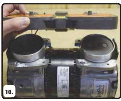
Check that orientation of the valve plate(s) with ports is correct and place over cylinders.
