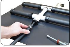
5. Slip hose clamp over the end of the tubing and push tubing onto the fitting.
