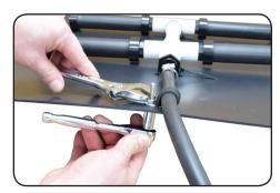
7. Attach strain relief fitting to the underlay plate. Use 17.5mm clamp for 3/8" tubing or 25.5mm clamp for 1/2" and 5/8" tubing.
