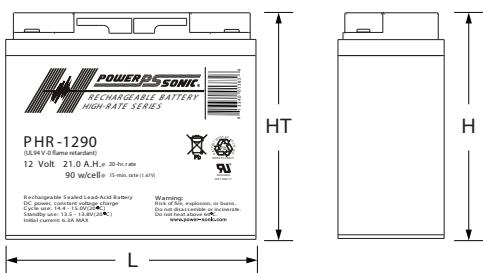
Tolerances are +/- 0.04 in. (+/- 1mm) and +/- 0.08 in. (+/- 2mm) for height dimensions.
