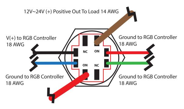
12V~24V (+) Battery Positive In from Fuse Panel 14 AWG
