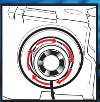
4. Secure the bulb by rotating lamp body and locking bulb into lamp body.
