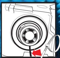
5. Fasen the black box with zip ties. Ensure there is no strain on the wires.
