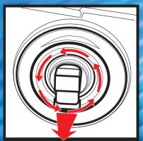
2. Disconnect the power line to the bulb. Rotate the bulb body to unlock from the lamp body.
