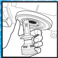
3. Remove OEM Halogen bulb. Install the F23-Series bulb into the lamp.
