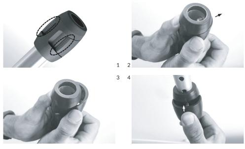
Grasp the clip of the Snap-Lock on the grip surfaces with one finger each. Press with both thumbs away from the pipe perpendicular to the pipe axis to open the clip. To close, light pressure from above onto the clip and snap it into place. !!! When assembling and disassembling the trailer there is on the moving parts and the snap-locks danger of pinching for fingers and hands !!!
