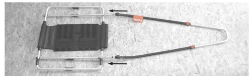
Use the two drawbars and the drawbar extension for mounting. Make sure that the bar with the reacha logo is on the right side (1). Insert the drawbar extension with the holes facing upwards into the orange snap-locks of the bars.
