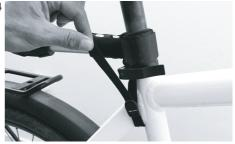
Place the Velcro strip of the Bike-Connector around the seat post at the desired height. Thread the Velcro, strip through the loop of the Bike-Connector, tighten it so strongly that the Bike Connector cannot slip and close the Velcro strip. Fix the Bike-Connector in the height with the help of the tension strap, by attaching it downwards around a suitable bicycle frame component.
