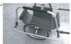
Open the snap-locks on the bow and first plug it into the front bow connector. Plug the bow then onto the rear bow connector and close the snap-locks. The Bow is ready mounted.
