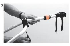
The Bike-Connector is pre-mounted on the drawbar extension. When attaching it to the seat post, make sure that it is aligned horizontally to the road depending on its later position. The length of the Bike-Connector should be adjusted so that the drawbar does not drag on the bicycle. Tighten all screws on the Bike-Connector so that it cannot twist (tightening torque 12 Nm).
