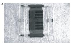
First insert the outer ends of one wheel frame into the connecting tubes in the trunk. Close the snap-locks at the desired hole position. The snap-locks are in the perfect position for correct locking when exactly half a hole is visible. It is best to leave the snap-locks open until the drawbar is attached, as this will allow the frame to be more flexible and the tubes to attach more easily. Attach the second bike frame in the same way.
