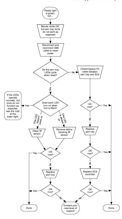
A steady green Ready light indicates that the controller is operating normally. If the pen tray failed or isn't communicating with the controller, your interactive whiteboard will still operate in mouse mode.
