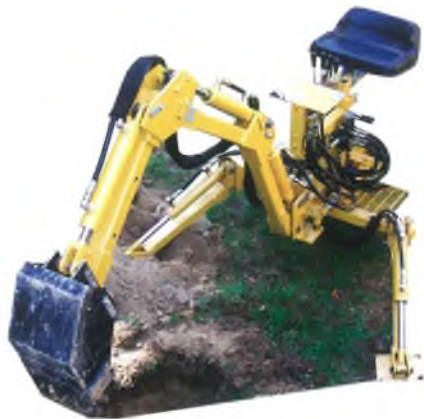
Mark DeGroot's Model 508 with Super Boom and Hydraulic Stabilizers
