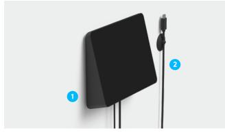
In-Wall Cabling: Supports Tap's rear and bottom cable exits so 3 you can route cabling either within or down the wall.
