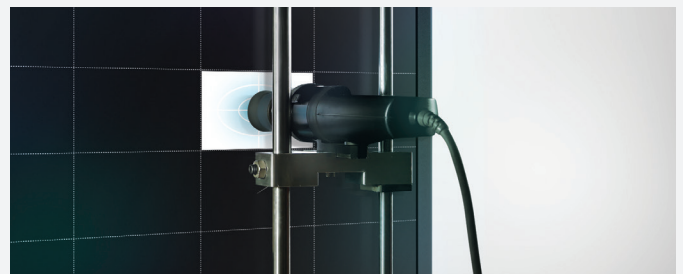
Figure 1. Samsung's multistep factory tuning helps ensure uniform brightness and color across video wall displays.
