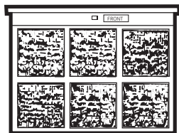
Dirty filter— Needs cleaning
