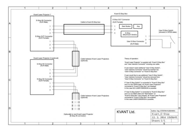
The E-STOP Remote is an integral part of the laser projector. It is there for the safety of the public as well as the operator. Modifying or using anything other than the E-STOP Remote provided, in the manner it was intended, may invalidate your laser projector's variance.
