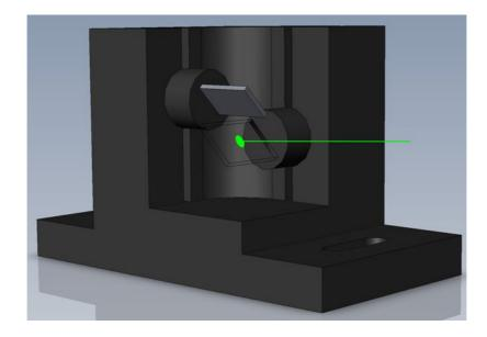
If not, use dichroic mounts DF4 to adjust the beam path accordingly (diagram below). To adjust the dichroic mount use the two adjustment knobs – each works for one axis.
