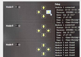
D: Start with the first dichroic filter (laser module1) and/or any other as necessary. Use the arrows associated with each module to move the beam to the desired position.
