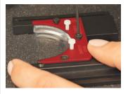
**3:** Put the front metal plate back in place and fasten it with the original 2mm countersunk hex socket bolts.
