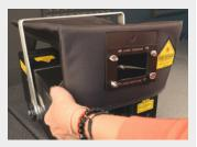
**2:** Push the rain cover under the attachment bracket.
