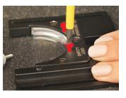
**4:** Gently tighten the two plastic screws to secure the lens firmly in place.
