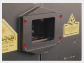
**2:** Fix it in position with four 2mm countersunk hex socket bolts.
