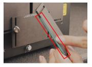
7: Place the top-wing of masking plate over both left and right wings, with its chamfered edge orientated downwards and towards the projector.
