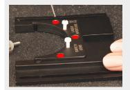
1: Use 2mm allen key to loosen three countersunk bolts that hold down the front metal plate of the bracket and remove it.
