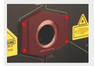
**1:** Use 2mm Hex socket key to attach DiscoScan bracket over the aperture.
