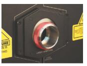
**4:** Bolt on the lens holder locking nut.
