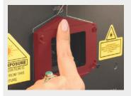
**1:** Place supplied bracket over the projector aperture, so it lines up with engraved lines.
