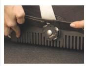
**7:** Make sure the side flaps of the cover stand away from the fan openings, so the airflow isn't restricted.
