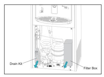
5. Attach the nut, the seal, and the elbow tube to the drain outlet and tighten it fully.
