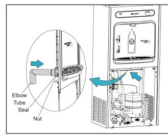
Connect one end of P-trap to the water drain tube and other end to the drain outlet. Note: P-trap is installer supplied part.
