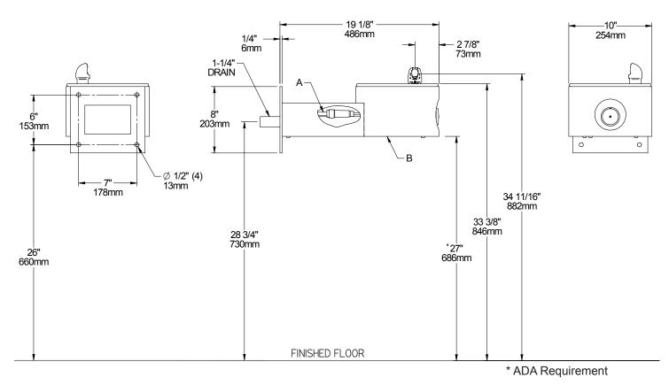
A = 3/8" O.D. UNPLATED COPPER TUBE CONNECT SHUT OFF VALVE BY OTHERS B = REMOVABLE BOTTOM COVER
