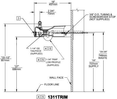
STANDARD INSTALLATION (FOR ALTERNATE 1311TRIMCA **INSTALLATION SEE SHEET 2.)**
