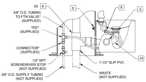
\*NOTE: TEE SHOWN ASSEMBLED FOR REFERENCE ONLY. POSITION TEE AND TRIM TUBING AS NEEDED TO FIT INSTALLATION APPLICATION.
